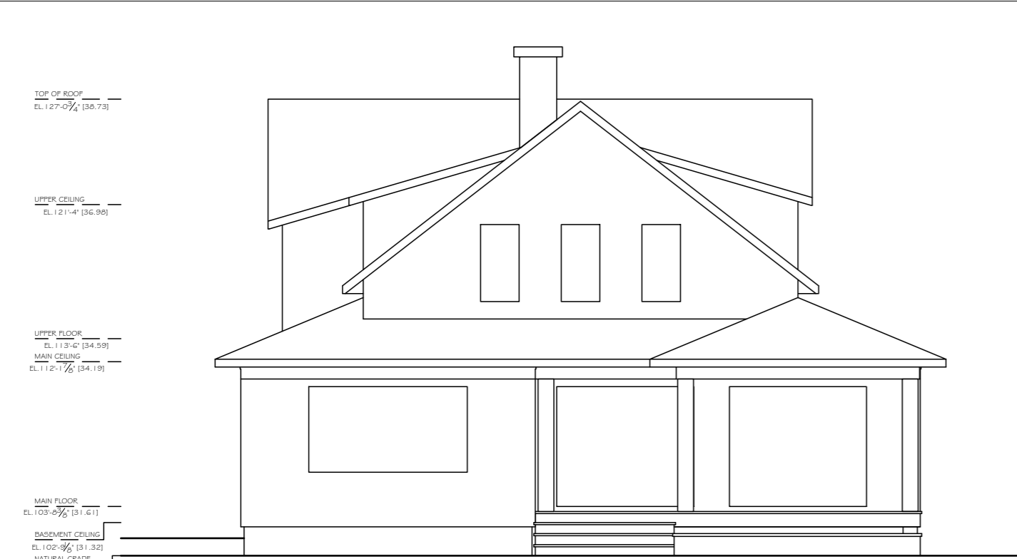
EAST ELEVATION — BASEMENT SLAB EL. 94'- \frac{3}{8} " (28.73)
