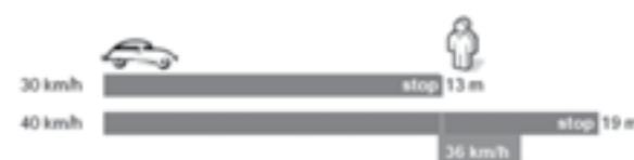
Figure 2 – Braking distance and speed of impact at 30 and 40 km/h
