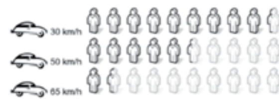
Figure 1 – Survival chances for pedestrians according to the speed at time of impact
