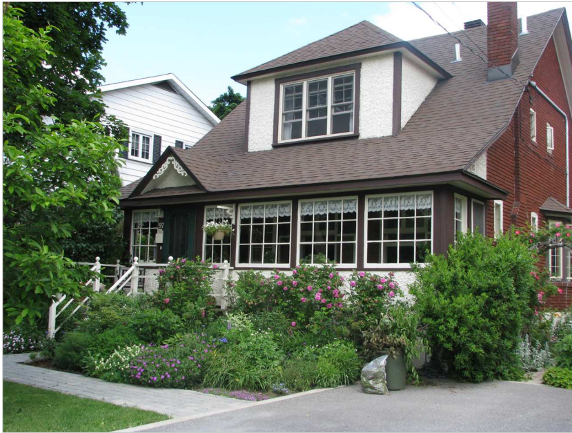
This shingle style Arts & Crafts house has been renovated to showcase its typical architectural features: sash or double windows; large windows on the veranda integrated into the volume of the shingled roof; stucco siding and woodwork that complements the bricks.
