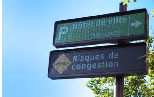
Figure 5-2 Dynamic parking guidance and information system
